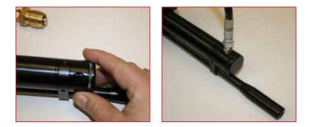
2) When charging is complete, bleed the excess air using the fill apparatus bleed screw and remove the fill adapter from the rifle. When finished, rotate the protective cover to prevent contamination of the fill port.
