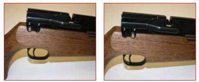
In addition to the safety catch, a loaded and cocked rifle can be made safe by decocking (uncocking). To decock the rifle, first pull the sidelever back to the rear position and remove the magazine. <u>While holding the sidelever</u>, squeeze the trigger and let the lever return forward under your control. The rifle is now decocked.
